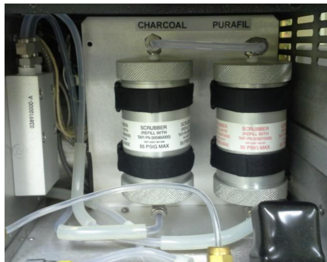
Fig. 2: Columns filled with charcoal and purafil inside the T701H.
