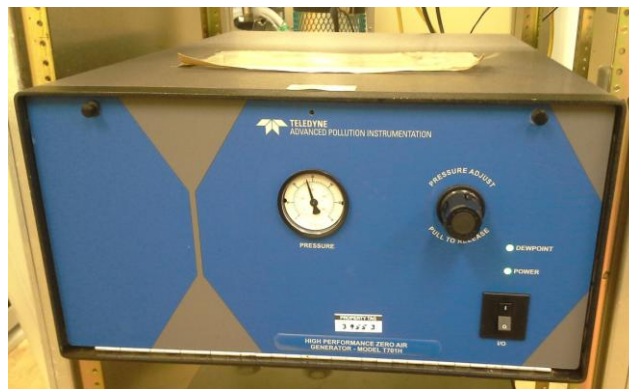
Fig. 1: Front panel of the T701H Zero Air Generator.
