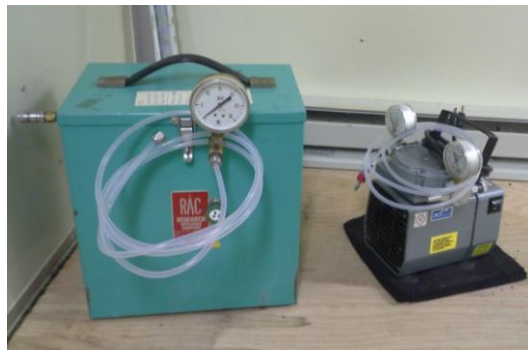
Fig. 4: Two part Audit Zero Air supply set up.
